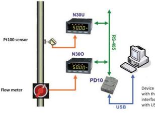
Device connection with the RS-485 industrial interface to the PC computer with USB interface.
