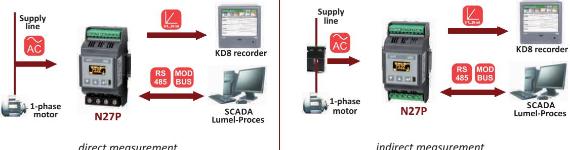
Conversion and recording of current engine load and energy consumption.
