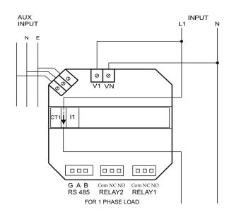
It is recommended that the wires used for connections to the instrument should have lugs soldered at the end. That is, the connections should be made with Lugged wires for secure connections. The Maximum diameter of the lug should be 7.0mm and maximum thickness 3.5mm. Permissable cross section of the connection wires <=4.0mm<sup>2</sup> single wire or 2 x 2.5mm<sup>2</sup> fine wire.
