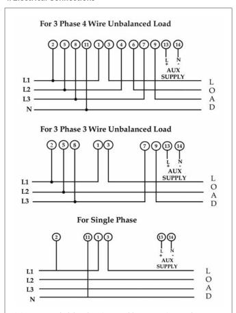
It is ecommended that the wires used for connections to the instrument should have lugs soldered at the end. That is, the connections should be made with Lugged wires for secure connections. The Maximum diameter of the lug should be 7.0mm and maximum thickness 3.5mm. Permissable cross section of the connection wires: <=4.0mm sqr. single wire or 2x2.5mm sqr. fine wire.
