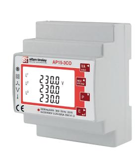
**Sifam Tinsleys AP15-3CO** is a new generation modern design power monitor that will measure and display electrical power quality parameters. It has been engineered to cover most applications (Single Phase and Three Phase networks / Built in Pulsed and RS485 Modbus / Import and Export kWh), replacing the need for several different models of this power meter.
