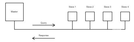
In the MODBUS Protocol the master can address individual slaves, or, using a special "Broadcast" address, can initiate a broadcast message to all slaves. The AP25-1DO Digital meter do not support the broadcast address.
