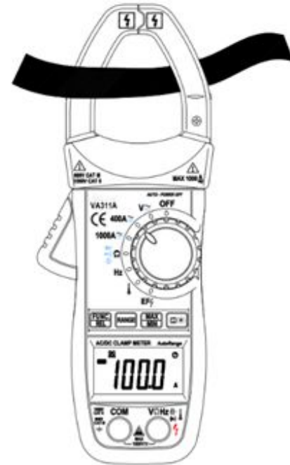
Figure 3-2 Measuring AC And DC Current
