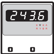
Screen 8 : System Voltage max Value. Value displayed after "Hi" flashing on Display
