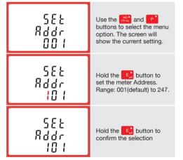
Use the Rest and Rest buttons to choose the necessary number, then press the St button to move along to the next number. To save the new setting, hold the St button for 3 seconds until the selection stops flashing
