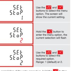
On completion of the entry procedure, hold the for 3 seconds until the selection stops flashing
