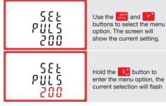
Use the we and P buttons to choose the desired pulse rate. To save the new setting, hold the E button for 3 seconds until the selection stops flashing
