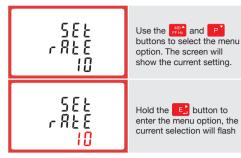
Use the with and without to choose the desired pulse rate. To save the new setting, hold the circle button for 3 seconds until the selection stops flashing
