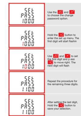
Hold the MA button for 3 seconds to exit the set up menu.
