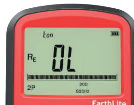
Fig: Overload Indication
